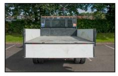
Ford Transit 350M 2.4TD (125ps) One Stop Shop 2.8m 1-way Tipper Ladder gantry; Top & bottom hinged tailboard. Double skin aluminium sideboards. Thermoplastic rear wings. 8 floor mounted flush fitting load lashing rings, rope hooks to bearers. Balance of Manufacturers Warranty applies to June 2015/ 100,000 miles.
